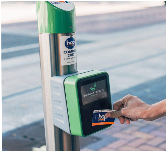
A TriMet Hop Fastpass validator placed curbside to facilitate off-board fare payment for MAX Light Rail. Individual small, pole-mounted validators require less upfront investment than curbside ticket vending machines in use on SBS routes. However, they offer less functionality such as obtaining or refilling transit cards. Image: TriMet.
